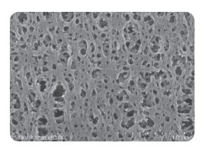
GVS hollow fiber membrane made of modified polyphenol is an asymmetric structure, the membrane layer is dense, and the outer layer is relatively open. Its unique structural design can result in lower bioburden, lower non-specific adsorption, faster filtration rate, higher throughput, and shorter filtration time, so it is very suitable for the pharmaceuti-cal and food industries.
